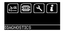
Connect the MAT Tool to a vehicle using the 16 Pin Diagnostic plug. The MAT Tool will then power up and take you to the Main Menu screen.
